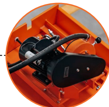
Avance ajustable de la sierra a 0.6 m/min
